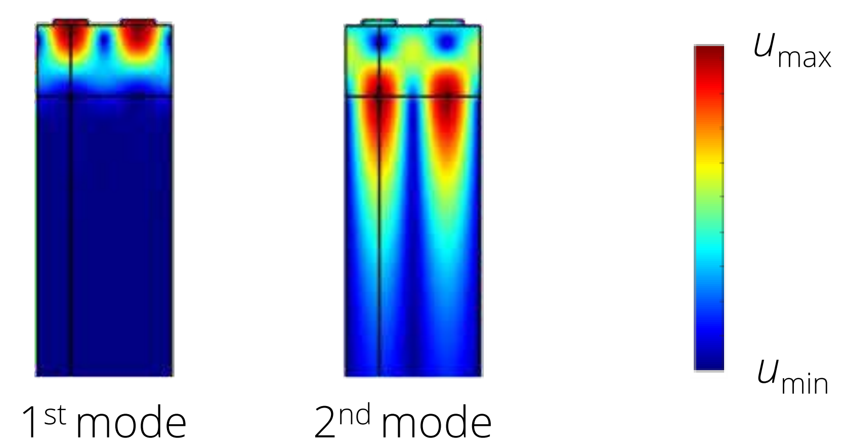
Figure 4: Exemplary eigenmodes of motion for antisymmetric Rayleigh-type (1 st ) and Sezawa-type (2 nd ) wave modes with u : total displacement.
